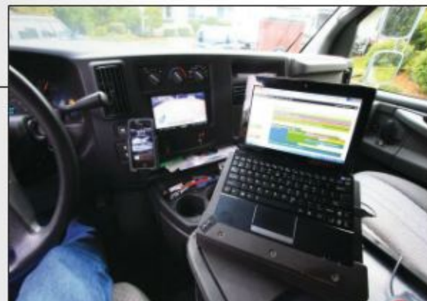
Every ADC Mobile truck has a full mobile office, with navigation, rear camera, Internet access, online scheduling and smartphones for instant communication between every installer.
