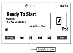
"Track Seek ▶1" or "Track Seek № " (on the radio or steering wheel) switch to next available channel.
