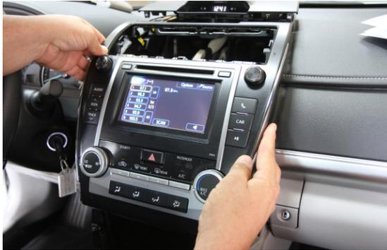
**2** Unplug factory 16 pin plug and plug into female end of T-Harness. Plug male end of harness into rear of radio. Connect camera RCA cable to T-Harness.
