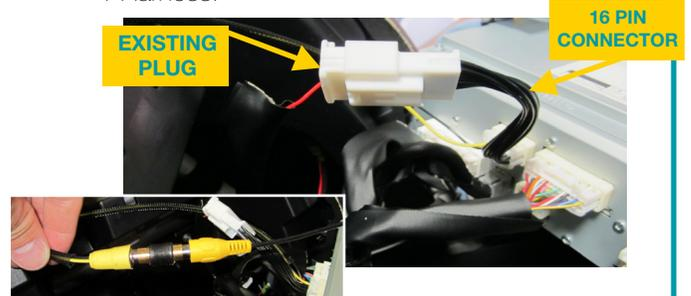
**3** A. Connect camera Red wire to suitable ACC or IGN +12V. Ground camera Black wire.
