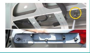
Use foam gasket to determine camera 9 mounting location on the drivers side. Drill a 19mm hole, mount camera & secure with nut.
