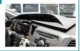
Remove 5 Phillips screws that attach multi-media screen to vehicle.
