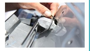
11 Connect the 2 wires located next to camera connector plug, Green (Parking Lines) and White (Image Flip) to corresponding color wires. Connect the camera cable.
