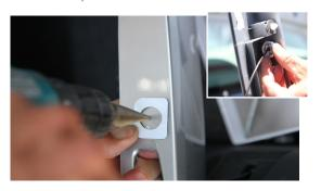
10 Unclip license plate light and route camera cable through opening. Remount light and re-attach trunk lip bezel.
