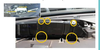
Remove 3 plugs from rear of multi-media screen. Plug in Factory Connect T-Harness into screen and reconnect all plugs. Route RCA and reverse trigger wire down to drivers kick panel.
