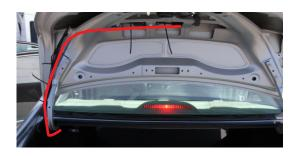
12 Check installation by putting vehicle in reverse to make sure image is correct and factory (yellow) parking lines are on the multi-media screen. Reassemble all parts of the vehicles to complete installation.
